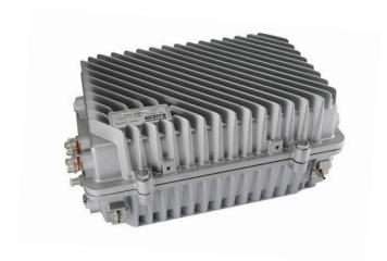
ACT RC3000 (Remote Multi-Access CMTS or Remote PHY Platform) is a series of DOCSIS 3.0 networking node device designed for next generation Node+0 and FTTX systems on top of the cost effective CATV coaxial network, delivering multi-media services into the multi-dwelling units(MDUs). RC3000 features three main components in one compact IP54 aluminium housing, Gigabit PON or Active Ethernet (P2P) ONU, optional HFC optical receiver node and remote DOCSIS 3.0 CMTS module.
