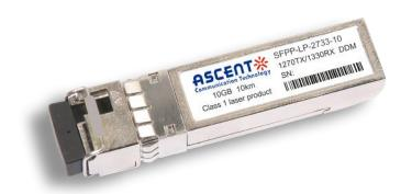
Ascent's SFPP-LP-XXXX-10 transceivers are designed expressly for high-speed communication applications that require rates up to 11.3 Gb/s. They are designed to be compliant with the SFF-8472 SFP+ MSA. The module is suitable for data links up to 10 km in distance over a  $9/125 \, \mu m$  single mode fiber.
