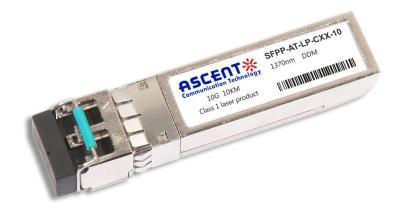
ASCENT's CWDM SFP+ transceivers are designed for use in 10-Gigabit Ethernet links with distances up to 10 km over single-mode fiber. These transceivers include a PIN photo detector diode and uncooled CWDM DFB laser transmitter. Digital diagnostic functions are available via an I2C interface. This module is designed for single-mode fiber and operates at wavelengths between 1270 nm to 1610 nm.
