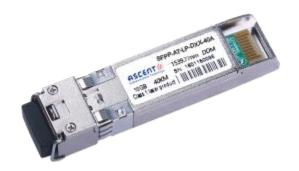
ASCENT DWDM ITU Channel SFP+ transceivers are designed for use in 10-Gigabit Ethernet links with distances up to 40 km over single-mode fiber. These transceivers include a PIN photo detector diode and temperature stabilized DFB-EML transmitter. Digital diagnostic functions are available via an I2C interface. This module is designed for single-mode fiber and operates at a nominal wavelength of 100 GHz ITU Grid, C Band DWDM wavelength.
