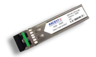
ASCENT's SFP-AF-LP-51-80 Small Form Factor Pluggable (SFP) transceivers are compatible with the Small Form Factor Pluggable Multi-Sourcing Agreement (MSA). The transceiver consists of five sections: the LD driver, the limiting amplifier, the digital diagnostic monitor, the DFB laser and the PIN photo-detector. The module data link up to 80 km in 9/125um single mode fiber.
