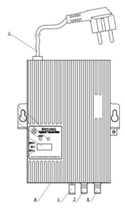
I: Optical signal input. When the device is working properly, the fiber port has an invisible laser beam. The fiber input port should not be looked at with a naked eye, so as not to cause accidental injury.
