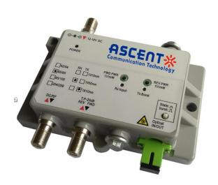
Ascent's RON1512 is a compact 1.2 GHz two-way node compatible with DOCSIC 3.1 FTTH architecture. It provides excellent forward and reverse path performance combined with high reliability and a user-friendly layout. RON1512 features an optical AGC function in the forward path to ensure the same RF output level in every home. The return transmitter has burst mode (turns on the laser by return signal) to greatly reduce return fibers.
