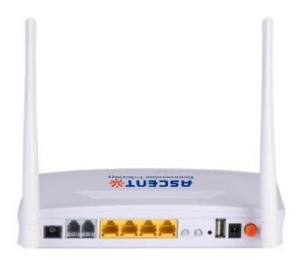
AP224S GPON HGU ONT is a GPON optical network unit designed to meet the requirements of broadband access networks. It is ideal for FTTH/FTTO applications to provide data, voice, and video services based on a GPON network.
