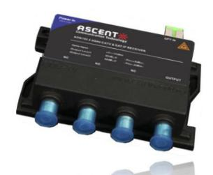
Ascent's AON120S 2.6 GHz CATV and SAT-IF Optical Receiver series is a cost-effective high-performance optical network unit which is designed and optimized to work in traditional CATV and satellite applications or for advanced triple play Fiber-to-the-Home (FTTH) architecture networks. The wide RF spectrum supports both the CATV spectrum and satellite IF spectrum up to 2.6GHz.
