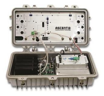
ACT AMAP3000 (Advanced Multi-Access Platform) is a series of networking node device designed for next generation Node+0 and FTTX systems on top of the cost effective CATV coaxial network, delivering multi-media services into the multi-dwelling units(MDUs). AMAP3000 features three main components in one compact IP67 aluminium housing, HFC optical receiver node, Gigabit PON or Active Ethernet (P2P) ONU and Ethernet over Cable (EoC) Master unit.
