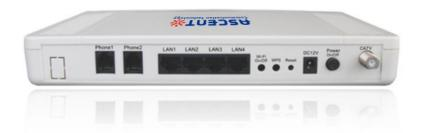
ACT AE200 P2P CPE is a series of high performance optical residential gateways designed to deliver high-speed internet connections, VoIP, IPTV, and traditional CATV services. AE200 provides network operators and services providers with the powerful residential gateway equipment needed to provide advanced services in Fibre to The Home/Business (FTTH and FTTB) networks.
