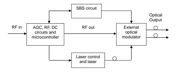
The RF signal enters the transmitter through the F-type connector on the rear panel, which feeds the AGC and RF sections of the transmitter. The RF section minimizes the CTB by producing CTB products of the same amplitude, but 180° out of phase with the CTB produced later in the modulator.
