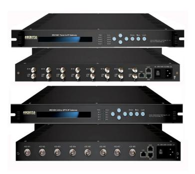
Ascent IRD1581 1RU Tuner (or ASI) to IP gigabits IP Gateway is a head-end interface conversion device which supports SPTSx256, SPTSx32, and SPTSx20 (for versions with BISS function) output. It is integrated with tuner demodulation (or ASI input) and gateway functionality, and can demodulate a signal from 8 tuners into TS and packet the TS into IP packages or directly convert the TS from ASI input into IP packages and output the IP packages through different IP addresses and ports.
