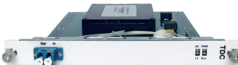
TDC tunable dispersion compensation module (A1600-TDC series)
