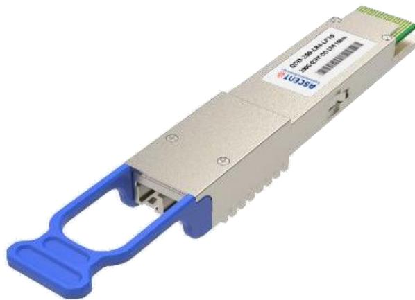
The ACT QDD-200-LR4-LP10 is a high-performance 200 Gb/s QSFP-DD optical transceiver designed for next-generation data center and service provider networks requiring high bandwidth and extended reach. Supporting 200GBASE-LR4 with four LAN-WDM wavelengths over single-mode fiber, the module enables reliable transmission distances of up to 10 km, making it well suited for data center interconnect (DCI), metro aggregation, and high-capacity enterprise applications.
