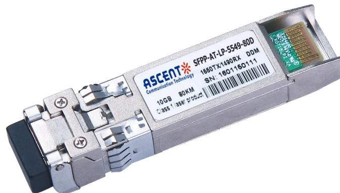
Ascent's SFPP-AT-LP-XXXX-80 transceivers are designed expressly for high-speed communication applications that require rates up to 11.3 Gb/s. They are designed to be compliant with the SFF-8472 SFP+ MSA. The module is suitable for data links up to 80 km in distance over a 9/125  $\mu$ m single mode fiber.
