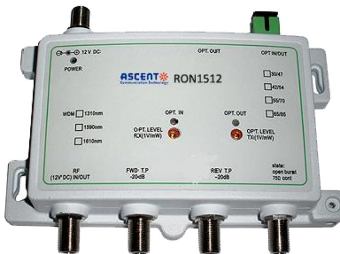
Ascent RON1512 is a compact, high-performance 1.2 GHz two-way optical node designed for DOCSIS FTTH architectures. Engineered for superior forward and return path performance, it combines high reliability, simplified installation, and a user-friendly layout. The integrated optical AGC automatically maintains a consistent RF output level in every home, while the burst-mode return transmitter activates the laser only when a return signal is detected.
