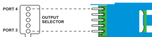
7-DC-xx-5-1218-WC directional coupler with cover has guides that only allow it to be oriented with port 3 as the tap leg. Remove the cover (blue) and rotate 180° as shown below to orient port 4 as the tap leg.
