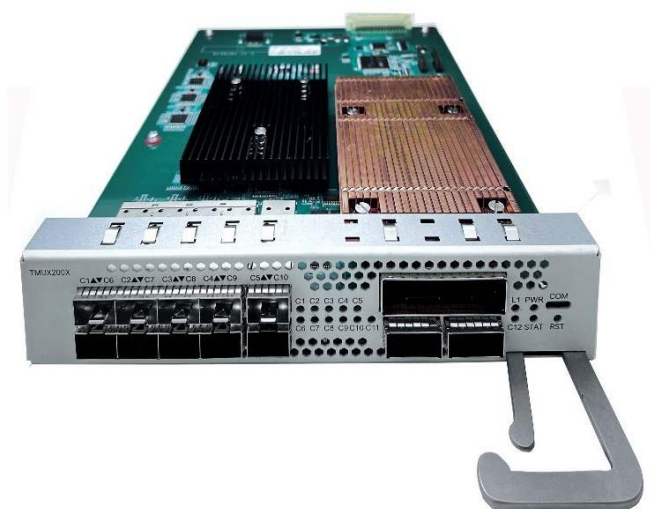
10*10G SFP+ plus 100G to 200G CFP2 DCO Transponder (A1600E-CFP2-10x10G)
