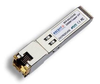
Ascent's SFP-AG-CO-02 10/100/1000BASE-T copper SFP transceiver is high-performance, cost-effective module compliant with the Gigabit Ethernet and 10/100/1000BASE-T standards as specified in IEEE 802. 3-2002 and IEEE 802.3ab, which supporting 10/100/1000Mbps data rates up to 100 meters reach over unshielded twisted-pair category 5 cable.
