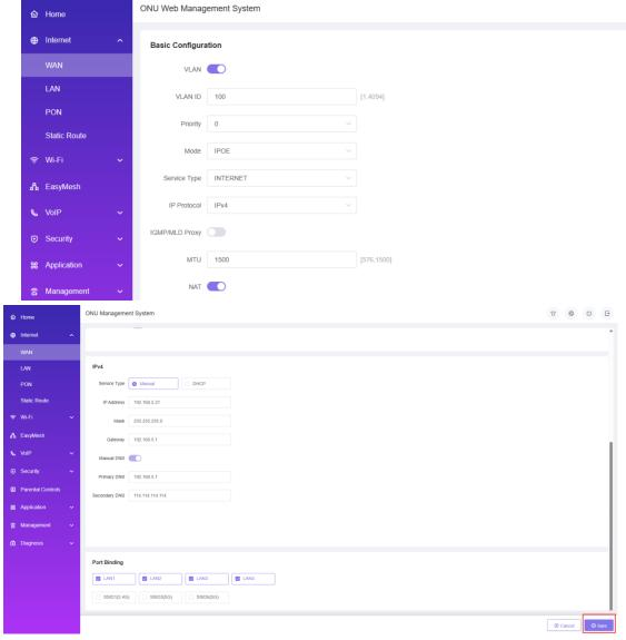
After configuring the parameters of Static IP WAN connection as below, click 'Sure' to finish the setting.
