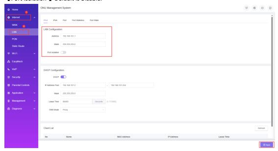
After configuring the parameters of LAN address as above, click 'Sure' to finish the setting.
