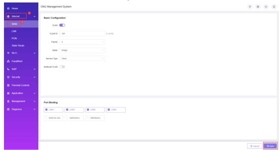
After configuring the parameter of Bridge WAN connection as above, click 'Sure' to finish the setting.
