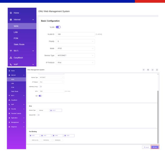
After configuring the parameters of DHCP WAN connection as below, click 'Sure' to finish the setting.
