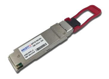
Ascent's 100G QSFP28 ER4 is designed for 40km optical communication applications. This module contains 4-lane optical transmitter, 4-lane optical receiver and module management block including 2 wire serial inter-face. The optical signals are multiplexed to a single-mode fiber through an industry standard LC connector.
