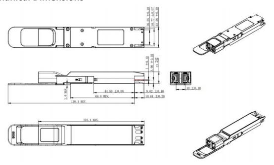
The optical interface port is a male Dual MPO-12 connector as specified in IEC 61754-7-1. Mates with two standard type MPO-12 female plug connectors with down-angled interface.
