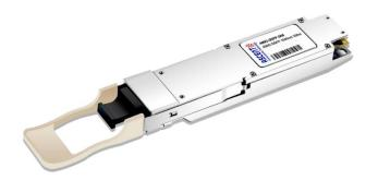
Ascent's 400Gb/s Octal Small Form-factor Pluggable (OSFP) full-duplex optical module offers 8 independent transmit and receive channels, each capable of 53.125Gb/s operation for an aggregate data rate of 400Gb/s on 100 meters of OM3 multimode fiber.
