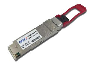
Ascent's 100G QSFP28 ER4 Lite is designed for 30km optical communication applications. This module contains 4-lane optical transmitter, 4-lane optical receiver and module management block including 2 wire serial inter-face. The optical signals are multiplexed to a single-mode fiber through an industry standard LC connector.
